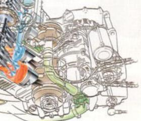
while the under-sides of the piston crowns are cooled by special oil-jets from the crankcase.
