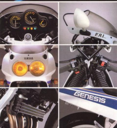
The full fairing has been aerodynamicallyproved at racing speeds. Extractor ducts in the fairing's sides take hot air away from the rider.
