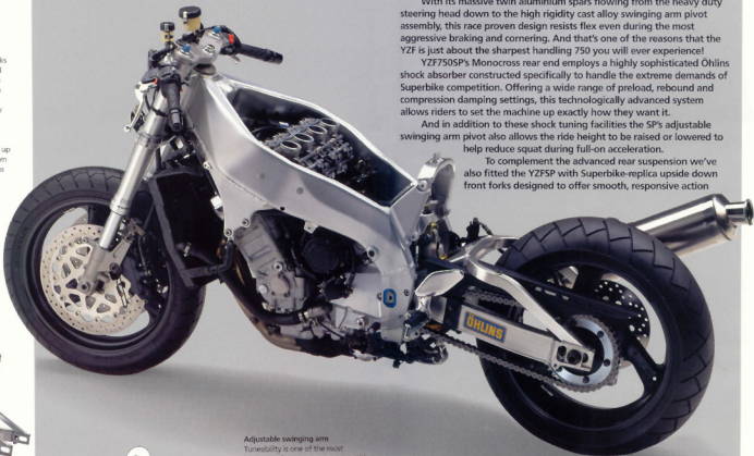
Front forks YZF750SP's advanced upside down front forks have been constructed using large diameter 41 mm tubes which are designed to resist flex when subjected to the intense forces generated by braking and suspension action. Together with the narrow pitch layout of the outer tubes this high rigidity front end delivers extremely precise handling at race speeds.
