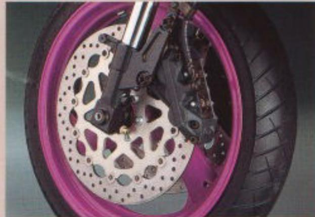
**Dual front discs with 6-pot calipers**
