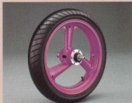
**Lightweight cast wheels/hollow axles**
