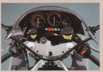
Manufactured from lightweight materials, the YZF's compact instrument panel features a central tachometer, easy-to-read speedometer, temperature gauge and indicator lights that keep the rider fully informed.
