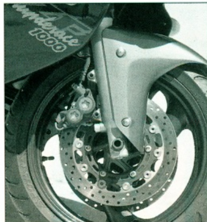
■ Yamaha fit all-new brakes to the YZF-1000R. The four-piston, one-piece calipers grab 298mm discs and offer outstanding braking power and feel.
