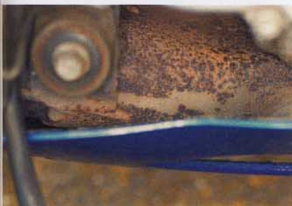
Top: The mileage is high, but not disastrous Middle: The rear shock is badly corroded and has lost its damping along the way Bottom: The silencer may look mint, but the pipes under the bellypan tell a very different story
