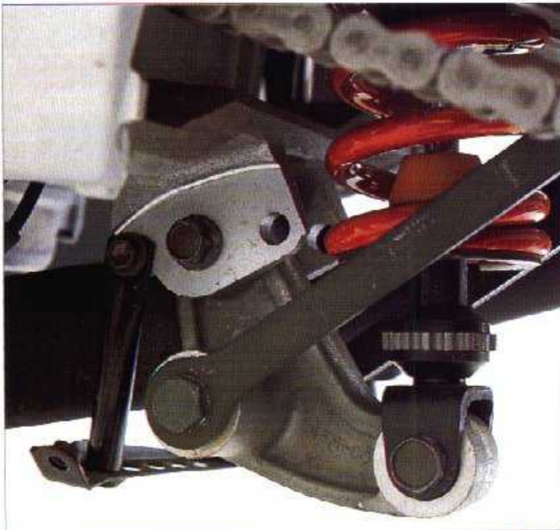
The Bilstein-type shock absorber is operated by a rising rate linkage system. No surprises here
