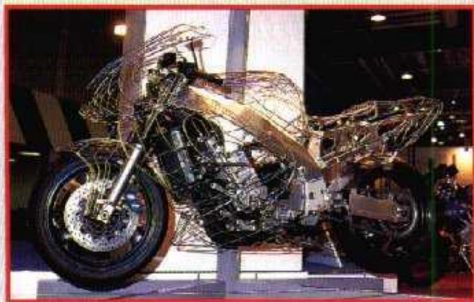
And here it is again – only this time stripped of plastic to reveal the all-new EXUP-based inclined parallel engine
