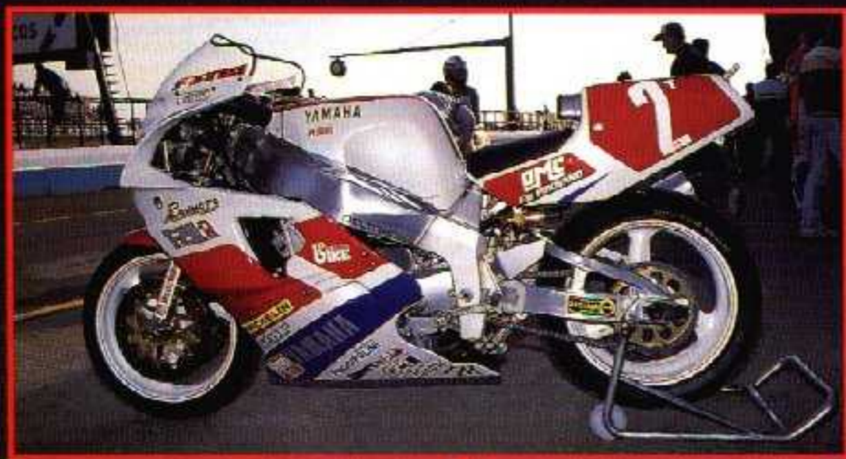
It was in 1989, with the FZR, that Yamaha introduced the aluminium Deltabox frame, using the motor as a stressed member
