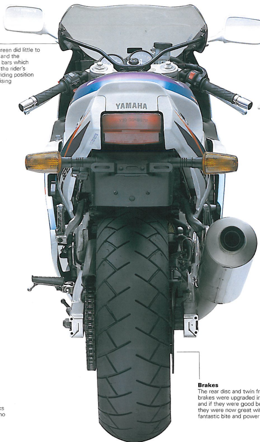
The four into one exhaust seen here came along with the 1990 model and over the years changed only in its finish
