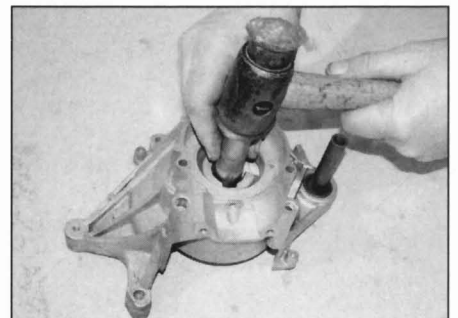
14.9 Driving a main bearing out of the crankcase
