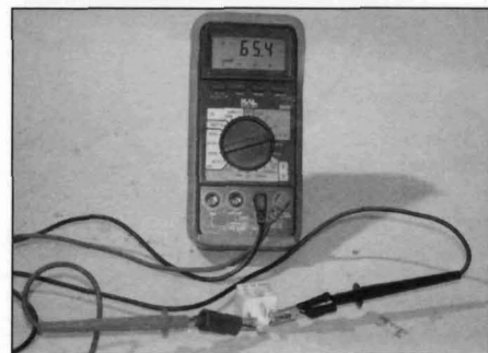
25.3 Measuring the starter relay primary resistance
