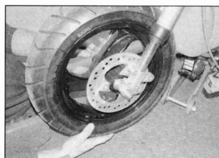
14.16c Support the wheel and withdraw the axle . . .
