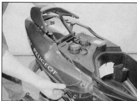
6.44 Ease the cowling off carefully
