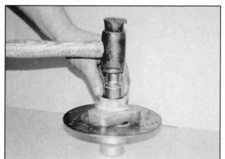
16.8 Installing a new bearing
