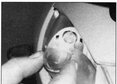
14.11a Unclip the bulb cover . . .
