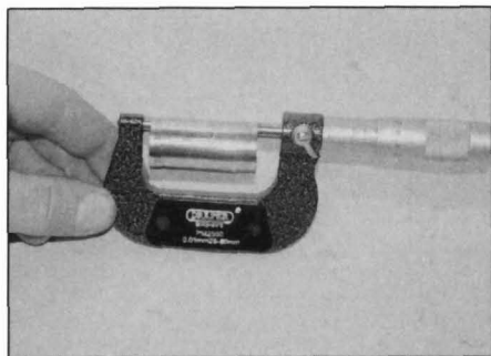
4.13 Measuring the length of the variator sleeve
