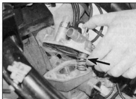
7.5 ... and remove the head with the thermostat and spring (arrowed)
