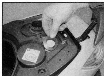
4.10 Remove the collars from the fuel and oil tank filler necks
