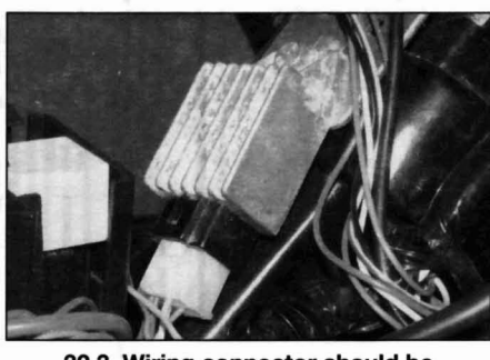
32.3 Wiring connector should be connected to the regulator/rectifier during voltage output checks
