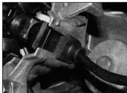
31.8b Wiring locates in slot in engine case
