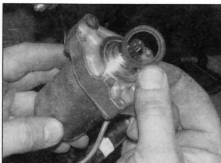
26.4 O-ring is fitted to starter motor body
