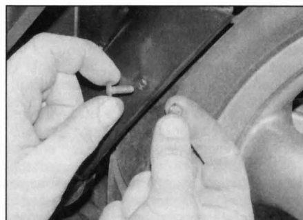
6.18 Mudguard is retained by two nuts and bolts on right-hand side . . .
