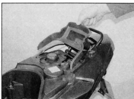
4.9 Remove the tool tray fitted to Speedfight models
