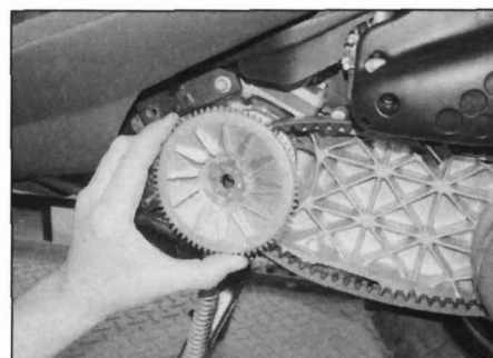
4.22a Install the outer pulley half . . .
