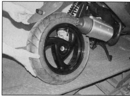
15.17b . . . and withdraw it from the machine
