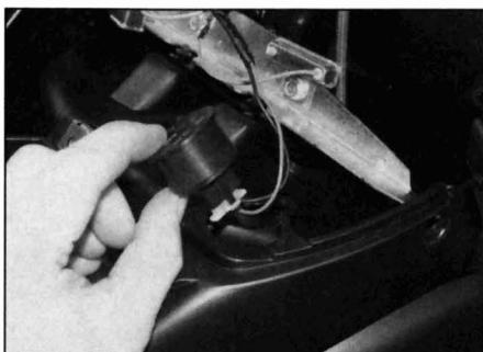
13.4a Relay location on Trekker . . .
