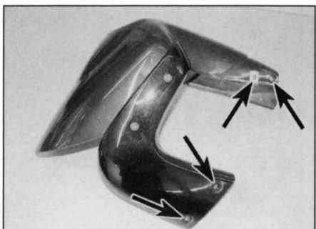
6.19 . . . and four screws on the left-hand side
