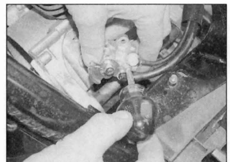
13.19b Bleeding a cable operated oil pump
