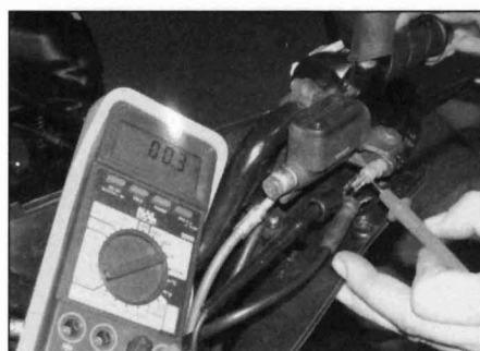
11.2b Testing the continuity of the brake light switch
