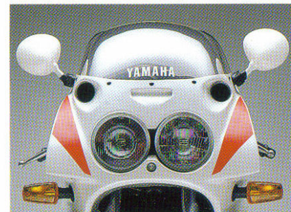
Sleek, aerodynamic fairing has been wind tunnel developed to improve high speed handling and increase top end speed. Twin FAI (Fresh Air Intake) ducts force cool, fresh air into the flat slide Mikuni carburetors for more efficient breathing and cylinder filling.
