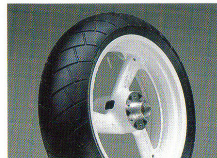
Lightweight alloy triple hollow spoke wheels are taken straight from our Grand Prix winning YZR racers. For 1990 they are fitted with new wider and lower profile Michelin Hi-Sport radial tyres to give even better traction.
