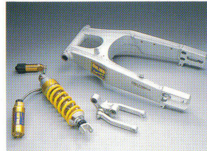
Fabricated lightweight aluminium Deltabox swinging arm keeps unsprung weight low and resists lateral flex forces. Race perfected Öhlins shock absorber and rising rate linkages ensure the rear wheel stays hard against the track surface even under flat out acceleration.
