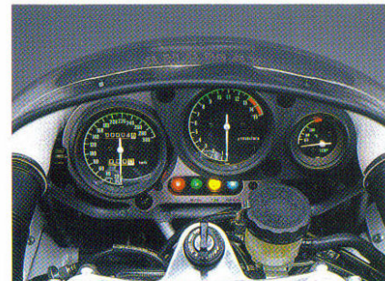
Instrument panel features centrally mounted electronic tachometer, water temperature gauge and easy to read speedometer for at a glance information. Oil, neutral, turn and high beam warning lights complete the neat and compact display.
