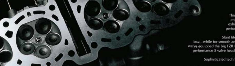
This is the most advanced supersport engine we've ever built. It produces exhilarating standing start and roll on performance. And it features Yamaha's innovative Genesis technology. Slant block layout keeps centre of gravity low-while for smooth and instantaneous throttle response we've equipped the big FZR with downdraft carburettors, high performance 5 valve heads and our unique torque boosting
