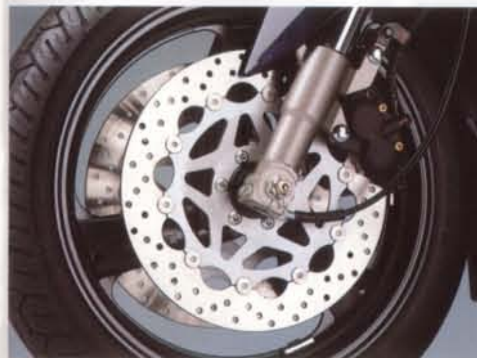
Front brake Phenomenal stopping power is supplied by the FZR's braking system which features twin 320 mm-diameter floating discs with 4-pot opposed piston calipers that bring the machine to a rapid standstill with minimum effort.
