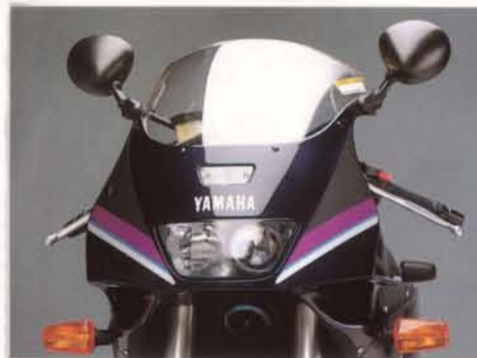
Fairing/FAI system The aerodynamically-efficient slant-nosed fairing slices through the air with minimal drag and incorporates a powerful flush-fitting headlamp assembly. Twin Fresh Air Intake (FAI) ducts force-feed cool air to the carburetors for maximum intake efficiency.
