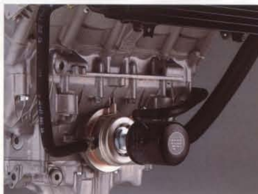
Radiator/Oil cooler The large-capacity radiator is situated in the area of maximum air flow to maintain constant engine running temperatures for optimum power output, and also dissipates heat from the liquid-cooled oil cooler.
