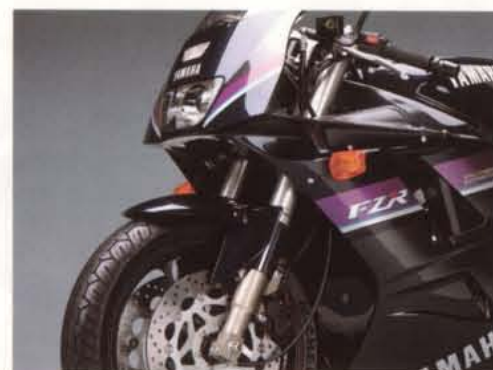
Front forks Developed from our Grand Prix racing programme, the FZR's upside-down forks use large diameter 41 mm tubes for maximum flex resistance as well as smooth damping action, and offer 120 mm of front wheel travel.
