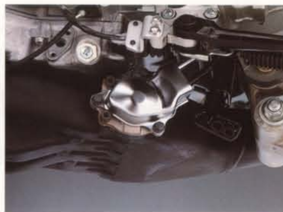
EXUP The FZR's Exhaust Ultimate Power Valve (EXUP) is operated by a microprocessor-controlled servomotor which constantly adjusts the exhaust's internal aperture to suit engine speeds, substantially boosting low to mid-range torque.
