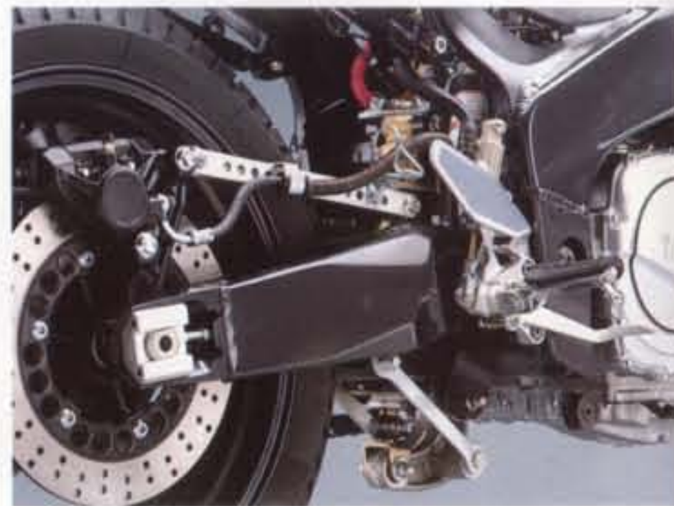
Rear suspension/Swinging arm The Monocross rear suspension system features a fully-adjustable gas/oil shock which gives 130 mm of rear wheel movement. Deltabox swinging arm keeps unsprung weight to a minimum and ensures maximum lateral rigidity.
