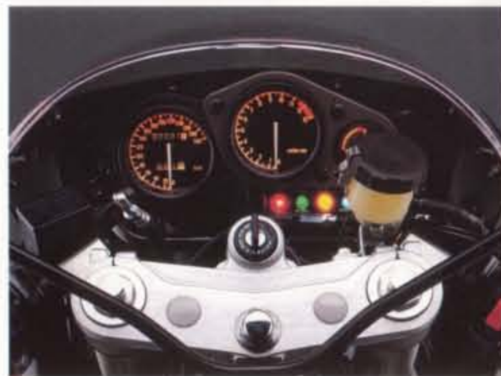
Instrument panel The centrally-mounted tachometer and temperature gauge hint at the FZR's racing heritage, while situated neatly on the left is the speedometer and integral tripmeter, with further information supplied by four indicator lights.
